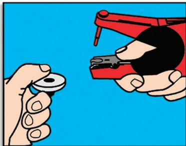
1. To load, depress spring clip and insert the female EID tag. Ensure that the raised portion of the tag, which encloses the transponder chip, is placed in the open portion of the jaws.
