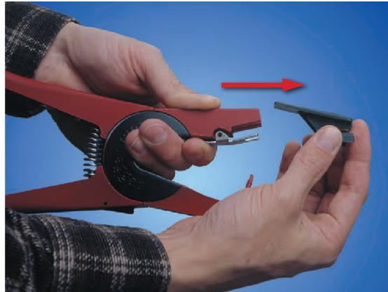
Use the red blunt pin and **remove the black insert from the base of the jaws** for applying EID tags, with red Universal Total Tagger or Retract-O-Matic™. The green Universal Total Tagger+ has a dark pin.
